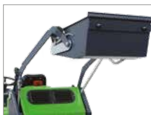
HOPPER PNEUMATIC DISCARGHE SYSTEM
